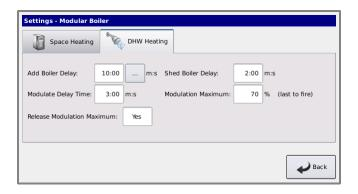
The example shows a 10-minute delay for the first boiler and increases by 3 minutes for each additional boiler.
