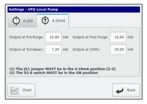
The 4-20mA output settings are all adjustable in 0.16mA increments.
