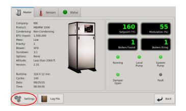
In the Bottom Left corner there is the Settings button which will allow changes to the operational settings of the boiler. See the Settings section.
