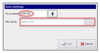
The next screen will display the files on the USB thumb drive. Select the settings file for the boiler.
