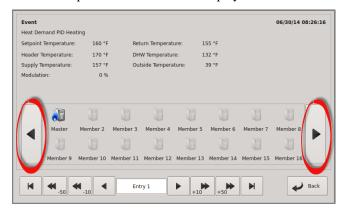
The Center middle shows icons of the boilers in the system/standalone with graphics indicating if they are firing. The large arrow buttons on the left and right of the boiler icons allow the viewing of the control state.
