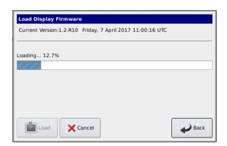
A pop-up box will tell you to remove the flash drive and select "OK". The display will reset and reboot with the new firmware installed.
