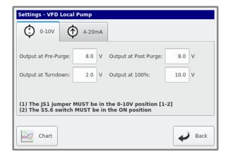
When JS1 is in the 0-10VDC position (pins 1-2), the output on J4 (J4.1+, J4.5-) will be a 0-10VDC signal and the settings on the 0-10V tab will be used.
