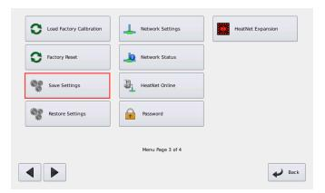
The default choice is, SAVE SETTINGS: To Location: "Onboard Memory". If the save button is selected the settings are saved and the control will verify by a progress bar.
