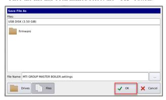
A verification box will appear with the File Name and location of the file. If all is correct select the "Save" button. The file will be saved to the thumb drive and return to screen 3 of 4.
