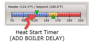
When the Header temperature is above the band (Yellow), the HEAT STOP TIMER (Shed Boiler Delay) is used to stop/shed boilers.
