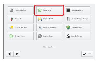
The *Local Pump Settings* Dialog is shown below. Set the *Local Pump VFD* to "*On*". This will enable the *VFD Pump Settings* button; press this button to open the VFD Local Pump Settings Dialog.
