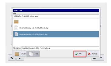
The current version of display firmware will be displayed, and the new version will be displayed. If the new firmware is correct select the "Load" button.
