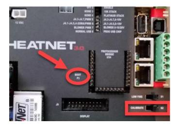
Boot P3 pins are located under the cover near the ribbon cable socket.
