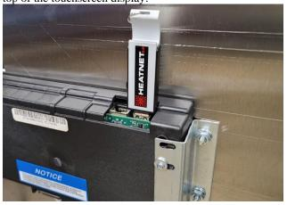
To ensure that a valid firmware file is always available on the HeatNet board, (2) file storage locations are available. A firmware file is loaded at the factory in both locations. This is to ensure that if a bad file is loaded by the user, the factory loaded file can be re-loaded to get the board functional again.
