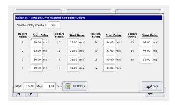
The same use applies to the DHW Start Timer (Add Boiler Delay) and DHW Stop Timer (Shed Boiler Delay) for DHW heating.
