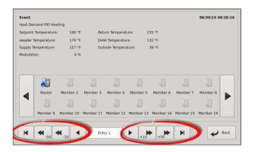
The top line, left corner indicates any condition that caused the event. This may be a fault (such as to indicate a sensor that has failed.) or general event as denoted by "Event". The top line, right corner displays the time and date the event occurred. In the bottom center of the command bar, the event # is displayed so that easy indexing can be done using
