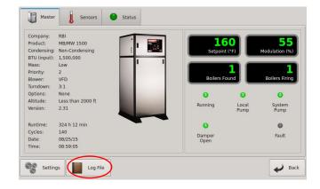
A new Filter Errors button has been added to the Log File Dialog.
