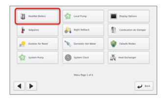
The *Boilers Settings* Dialog is shown. Set the *Limit Firing* value to the maximum number of boilers allowed to fire at any time. Setting the value to 16 (maximum number of boilers in a single HeatNet system) essentially disables the feature.
