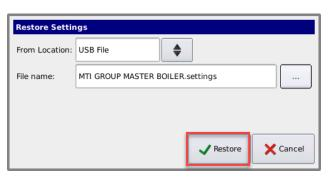
The saved settings will be loaded, the control will reboot, and the boiler will run with the new settings.
