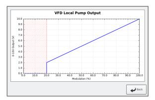
When JS1 is in the 4-20mA position (pins 2-3), the output on J4 (J4.1+, J4.5-) will be a 4-20mA signal when the boiler is running and the settings on the 4-20mA tab will be used. When the boiler is off, the output will be 4mA.
