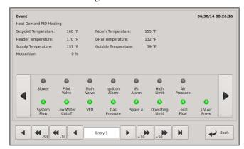
They are the Circulator Pump state, and the ignition condition (Main Valve, Pilot Valve, Blower, and the Ignition alarm). There are also indicators for interlocks and auxiliary functions.
