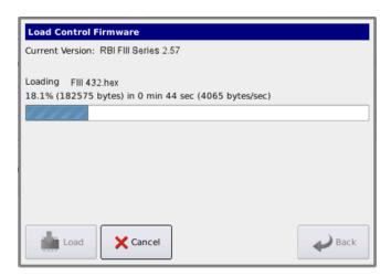
Once the firmware has been downloaded and the control rebooted, it now contains all of the default setting values. The settings should be restored. See Saving and Restoring Settings.
