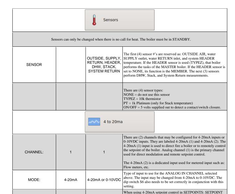
SOURCE. This is the temperature when a BOILER START signal
