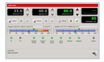
The Maximum value is used to set the maximum fire rate of the boiler. To adjust the Maximum fire rate of the boiler, press the Adjust button under the Maximum (%) value shown in the display. The percentage value will turn green. Then use the arrow keys to adjust the value up or down. Adjust it using the arrow keys and then press the green check key to save the value. Press the 'X' key to discard the setting.
