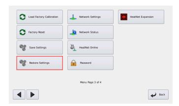
If you select "Onboard Memory", then "Restore". The saved settings on the control will be restored from the onboard memory.
