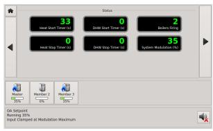
The above screen on the Master boiler displays the start and stop timers that are used to bring on boilers below and shed them above the heating band. When the Header temperature is below the band, the Heat Start Timer (Add Boiler Delay Timer) is started. Once it reaches 0, the next boiler will fire and be added to the Boilers firing display. This will continue until the Header temperature enters the Heating Band (Yellow) or all boilers have fired.
