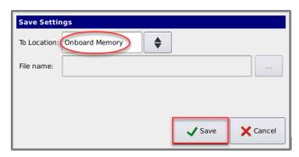
If an event destroys the control, all settings are lost. A servicing technician does not always know how the boiler was set up. Having the settings saved on a thumb drive on site allows the settings to be restored to a replacement control board.
