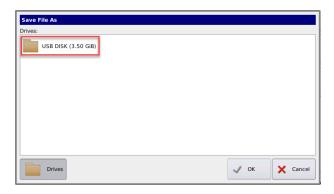
After selecting the USB Disk folder, any files and folders that are on the thumb drive will be displayed. Though you can't create a folder via the touchscreen display, if you have a folder you can choose to save the file there.
